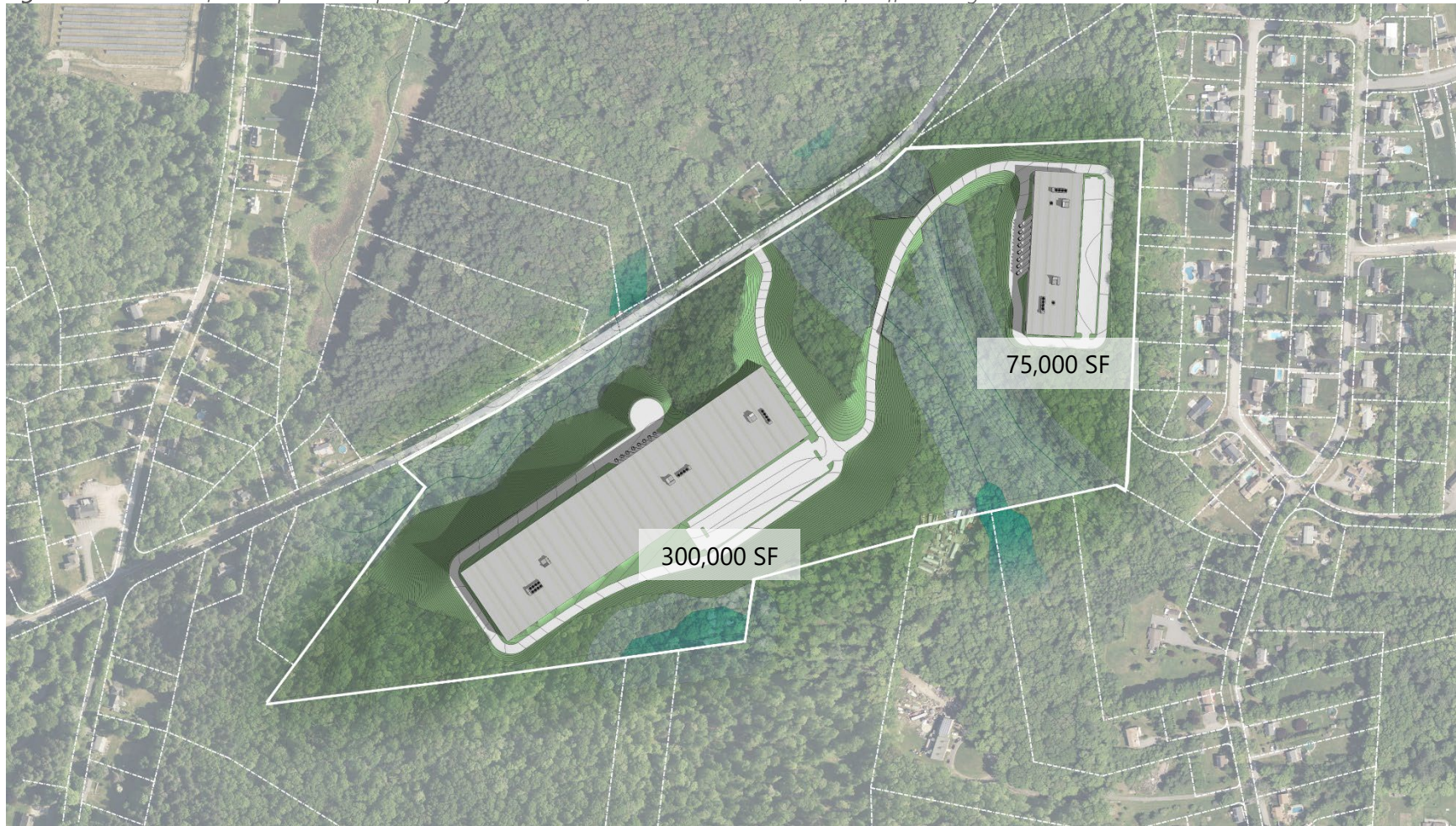
Figure 11. Plan view of Concept 1B with property outline in red, wetlands in dark blue, 100ft buffers in light blue
